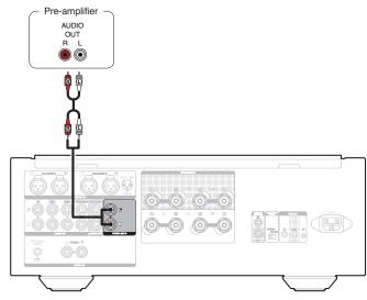
**1** Turn INPUT SELECTOR on the unit to select the input source to "POWER AMP".
